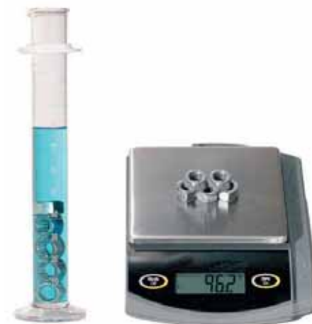
Figure 4.10: Use the displacement method to find the volume of irregular objects. Use a scale to find the mass.
